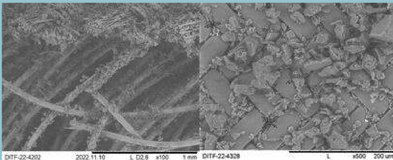
Left: Filter cake structure on 3D warp-knitted fabric cross-section, upstream side. Right: Microplastic particles on filter-woven fabric, upstream side. Images: DITF
